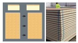
creates the recommended APA spacing. See illustration for guidance on orientation of boards. When cutting is necessary, make cuts on flush edges. Before packaging, the bundle is marked down the edge to designate the corner where adjacent sides contain non-flush edges. **NOTE: Due** to variations in wood dimensions and tolerances, as well as, uncontrollable ambient conditions that can alter wood dimensions at the time of installation, the proper overhang is not always present.
